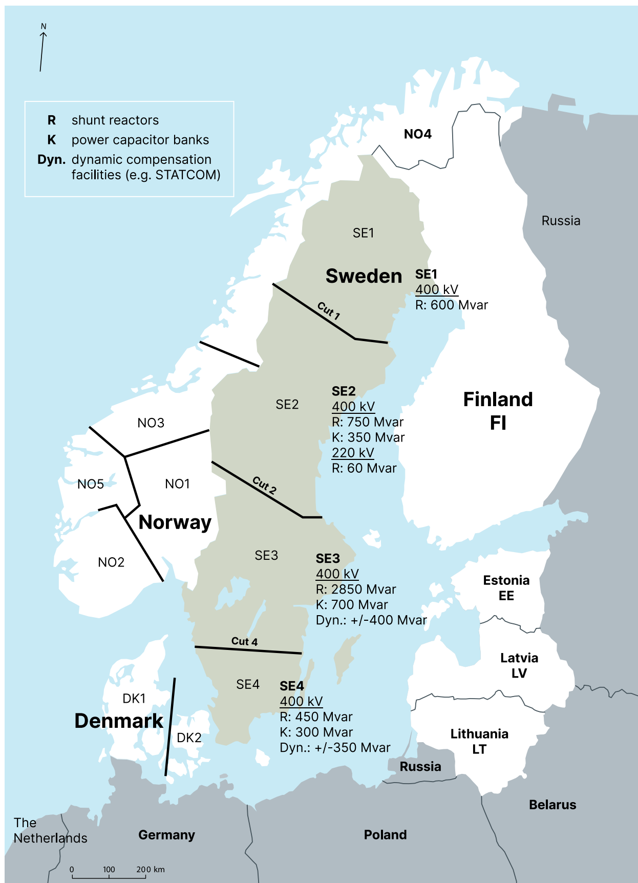
Figure 4. Planned investment in facilities for the compensation of reactive power (voltage regulating devices) in the transmission grid.
